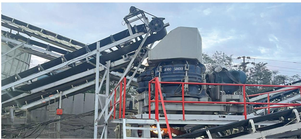
Taurian CB Series™ cone crushers were first introduced in 2019. They were introduced due to growing demand for product which is precisely to specification. The CB series™ features a unique roller and taper bearing design, along with hydraulic cylinders to maximise clamp down pressure. These dependable and powerful crushers excel in both quarrying and mining applications, making them a perfect solution for high-demand operations requiring precise crushing performance.
