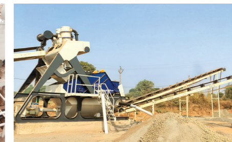
Rajasthan | Dewatering Screen
